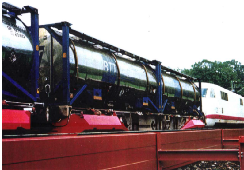
figure 8 shielded system with body shrouds at the locomotive and low noise barriers at the track
